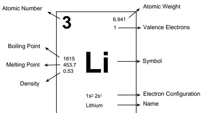
Note that for this element, lithium, the atomic number, atomic weight, valence electrons, symbol, electron configuration, name, density, melting point, and boiling point are all given in a single box. Most tables have a key that identifies the information included in the table.
