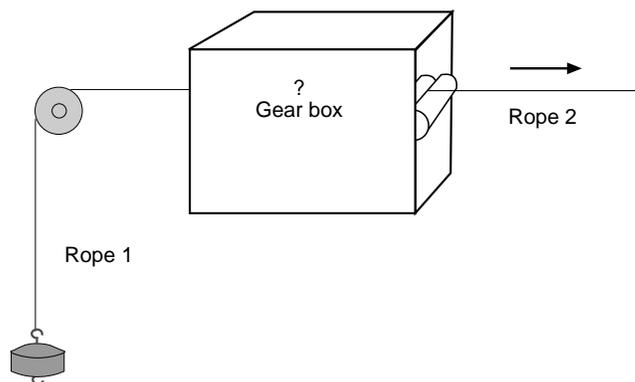
Assume there is no loss of energy doing work against frictional forces and that there are no sources of energy involved except for the forces pulling on the ropes. If a force of 6.0 N is exerted on the first rope, what force would be exerted by the second rope and why?
