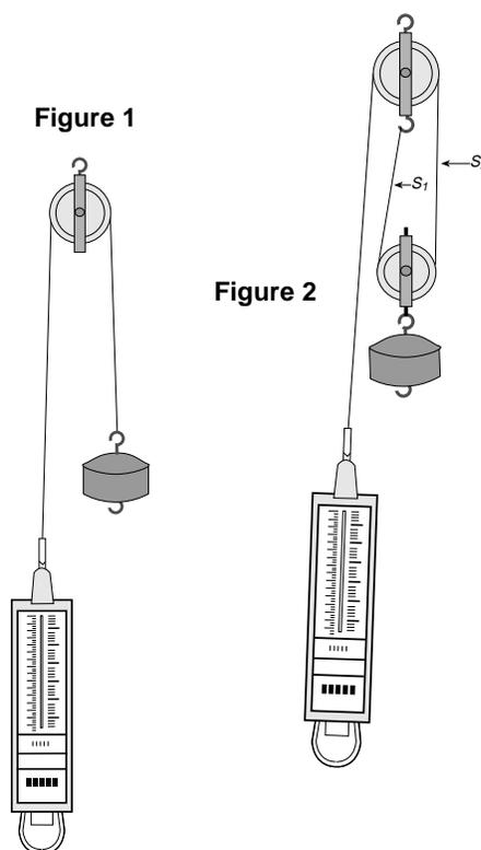
moved doubled and the force on the spring balance was reduced to half, so that the force multiplied by the distance the spring balance moved was the same as that for the one-pulley arrangement. This corresponds to the amount of work done in lifting the mass hanging from the pulley.
