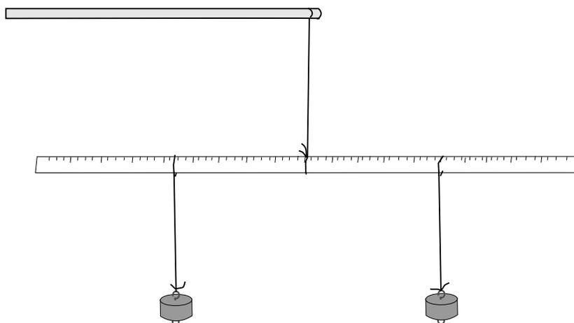
It is recommended that students explore this phenomenon further by placing a prism or other appropriately shaped object *under* the meter stick to serve as a support and placing the masses *on top of* the stick. They then repeat the measurements using 30-g and 60-g masses.
