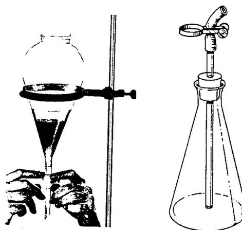
in a stoppered bottle. Separate the liquids by pouring them into a regular funnel fitted with a short length of rubber tubing and a clamp. If coffee is used, better results may be gained by first extracting the oil. Have students label the evaporating dish with name, time, and date.
