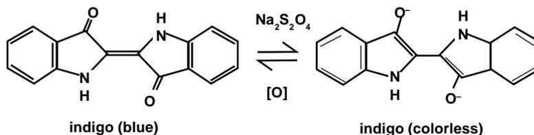
As long as the cotton cloth is in the solution, it stays white. As the “indigo white” becomes oxidized by the oxygen in the air, it turns blue. If a deeper blue color is desired, repeat the dipping and pulling out several times. Indigo is a vat dye due to this process. The denim used to make blue jeans is often dyed with synthetic indigo. This insoluble blue pigment is permanently bound to the fabric. Therefore it is called a fast dye.
