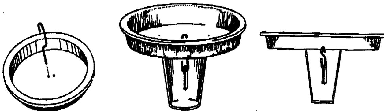
Bring a charged rubber rod (or charged side of a balloon) close to, but not touching, the pan. What happens to the strips of aluminum foil hanging from the paper clip inside the glass? Touch the pan with the charged rubber rod. What happens to the foil leaves? When you remove the rubber rod, what happens to the leaves?
