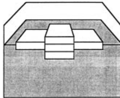
Figure 2. Addition of two wood blocks to simulate a mountain range.
