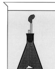
Flask of hot colored water in a beaker of cold water. Note relative position of glass tubes.
