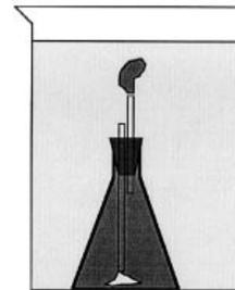
Flask of hot colored water in a beaker of cold water. Note relative position of glass tubes.
