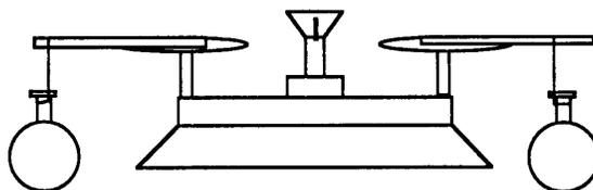
Using a pan balance. Place on the corner of a lab table so that flasks do not hit the table.
