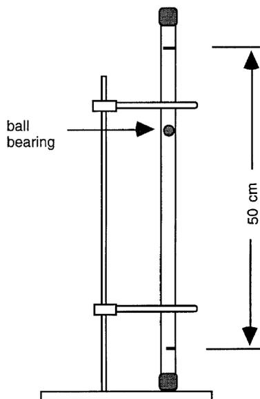
Figure 1. Laboratory setup for viscosity determination.
