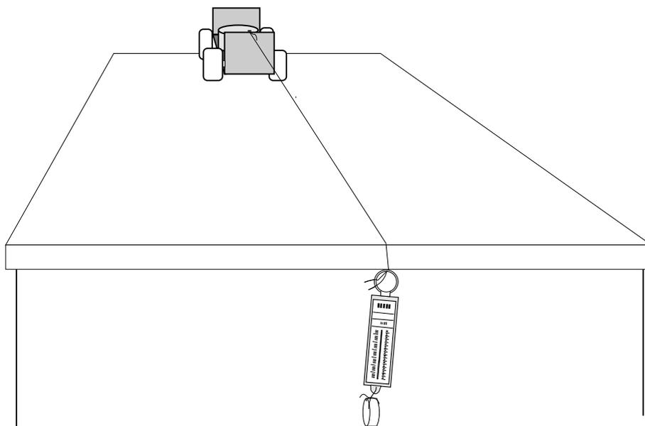
Students then release the cart, and it is set into motion by the weight of the mass hanging over the edge of the table. They should carefully observe the reading of the spring balance as the cart and mass accelerate, noting that the force the small hanging mass exerts on the cart, as indicated by the balance reading, hardly changes from its value when the cart is stationary.
