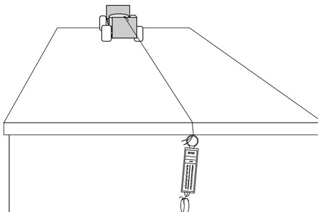
To get more meaningful results corrected for friction, calculate the slight extra force, if any, that was needed (in addition to the force for the empty cart) to pull the cart carrying the cargo. Use the spring balance to measure the right combination of small extra masses whose weight is equal to this extra force.
