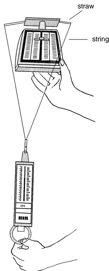
apply a force, the intention is to provide a further demonstration of the generality of Newton's third law by showing it applies even when the force on one object could be considered to be pushing it and on the other object to be pulling it.
