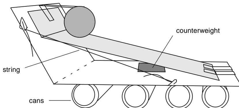
Tape holds the rubber ball in position at the top edge of the flap. Empty aluminum soft drink cans should be placed under the cardboard, so that the cardboard can roll on them. A counterweight near the center of the horizontal section of the cardboard keeps it from tipping over.
