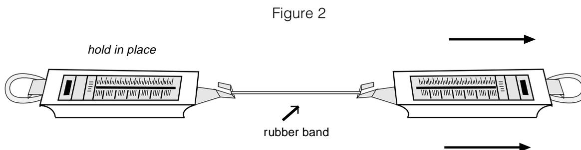
Ask students to try to make the force readings unequal. They should find that the two forces are always equal.
