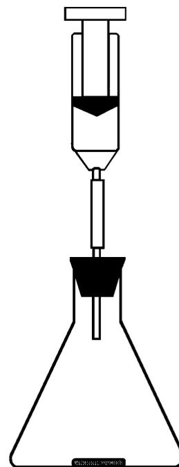
of the entire setup again (it should not change). Finally, they should remove the stopper, releasing the excess  $\text{CO}_2$ , and take the mass of the entire setup again. They should see a drop in mass that represents the mass of the  $\text{CO}_2$  gas.
